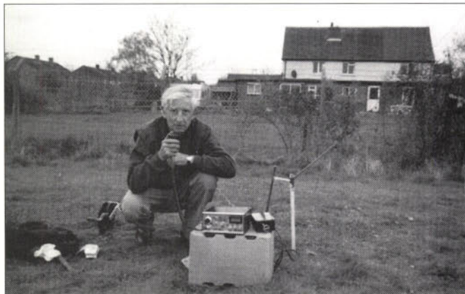
Fig. 1: 'Top Band' addict Pat Painting G3OUC, shown here with his 1.8MHz 'Skyliner 160' transceiver, flies kites to get his antenna to a good height (see text for further details).
