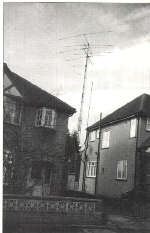
Fig. 2: Don McLean G3NOF, based in Yeovil, Somerset, has been reporting on h.f. operations to PW for many years. The photograph shows Don's (top of tower) TET HB33SP 3-element, middle is the Tonna 9-element for 144MHz and bottom is the Cushcraft A3WS 3-element antenna. Don's trapped dipole can also be seen mounted on the pole on the side of his house.
